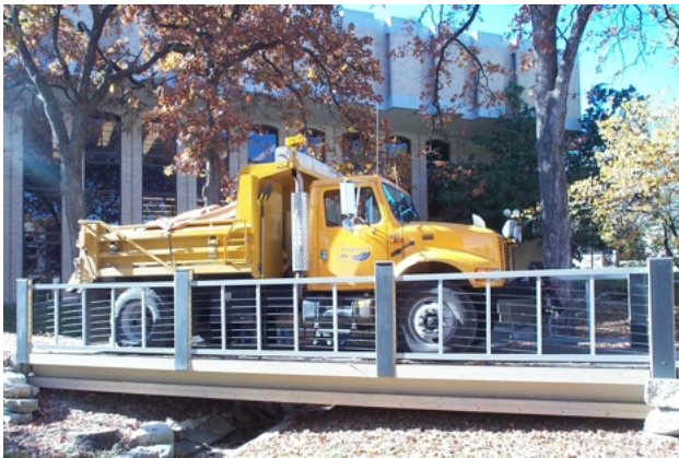
Load tests show that the SCB exceeds an AASHTO H20 highway rating.
