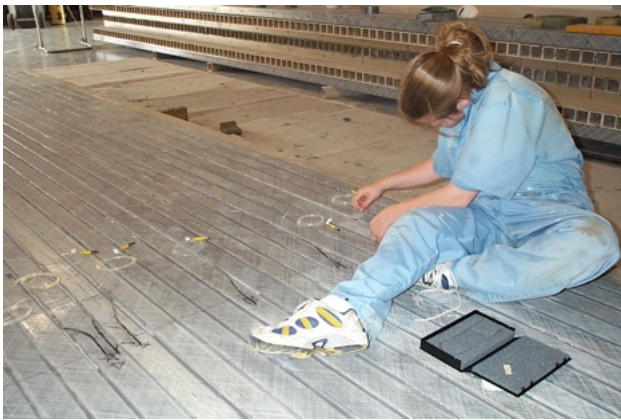
Fiber-optic strain sensors in the SCB were embedded during the off-site manufacture.
